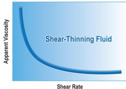
The viscosity of a grease changes when sheared. Apparent Viscosity, reported in centipoise, gives a design engineer an indication of the “shear quality” of a grease at specific temperatures. (Water is about 1 cP. Wood putty is about 1 million cP.)
